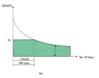
From this annual discharge curve, a truncation is made at a discharge Q which is the discharge corresponding to a time of 't' days, where t can be the median (say, 182 days or 50 percent duration, denoted by ( $Q_{182}$  or  $Q_{50\%}$ ), or a higher Q (t less than
