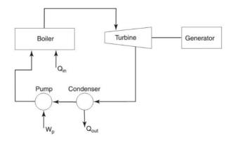
The schematic diagram also shows heat( $Q_{in}$ ) being supplied to the boiler and generator connected to the turbine for the production of electricity. Heat ( $Q_{out}$ ) is removed by the condenser and the pump supplies energy (Wp) to the feedwater in the form of a pressure increment to allow it to flow through the boiler.
