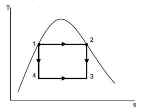
b)The carnot cycle is not a suitable model for vapour power cycle because it cannot be approximated in practice.
